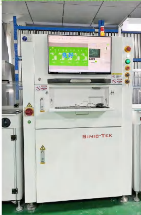
In-line solder paste inspection (SPI)
