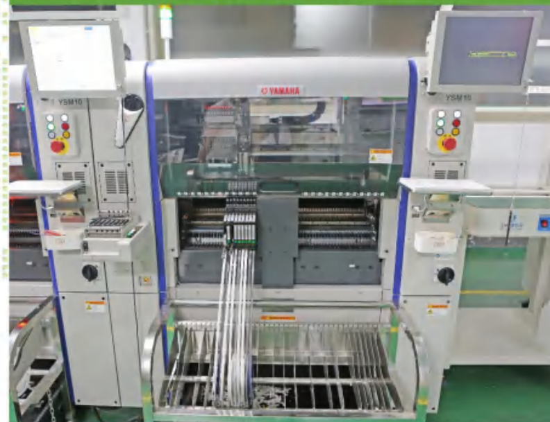
Latest YAMAHA placer with the most efficiency and precision (SMT)
